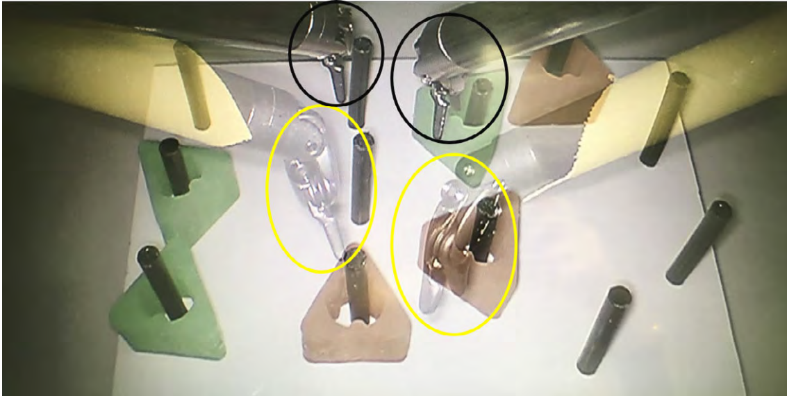
Figure 5.23: Augmented reality (AR) could be used to help surgeons learn and also perform minimally invasive surgery. In the sample scenario shown above, a trainee manipulates the real tools of a da Vinci robot (circled in yellow for visibility). This real tool view is overlaid on a pre-recorded stereoscopic view of an expert's instruments (circled in black for visibility), from which the trainee can learn.
