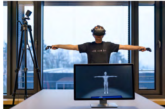
Figure 3.8: Our body models are now used for problems in psychology and medicine. Our SMPL body model captures realistic body shape and can easily run in MR/VR applications. We have recently developed simple methods where clinicians can create avatars using only the controllers of an HTC Vive.
