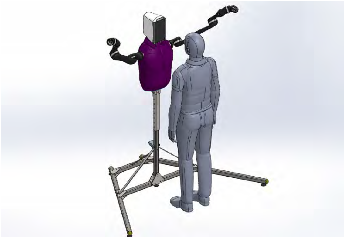
Figure 5.28: A CAD model of HuggieBot 2.0. This robot features two Kinova JACO 6-DOF arms, a customized v-shaped base for close interactions, an adjustable stand to adapt to user height, an inflatable pressurized chest to measure hug tightness, and a screen for showing either an animated face or a pre-recorded video message.
