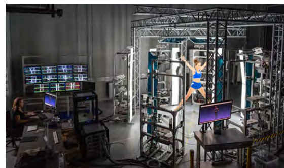
Figure 3.11: The 4D body scanner captures 3D meshes of the full body at 60 fps.
