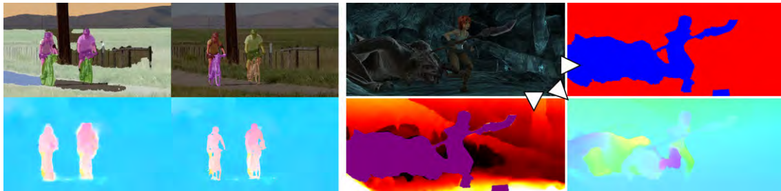
Figure 3.36: Reasoning about the structure of the scene improves optical flow estimation. Semantic segmentation helps to impose meaningful motion priors based on object identity (left). By segmenting the scene into a static background and moving objects an algorithm can use strong geometric constraints in the background region, simplifying the flow problem (right).
