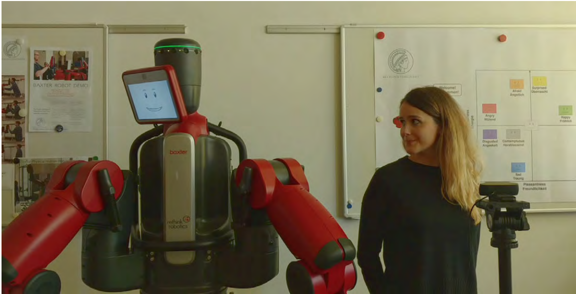
Figure 5.24: A human teleoperates the head of Max, our Baxter robot, via camera-based pose estimation and facial emotion recognition.
