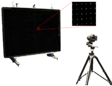
Figure 2.18: Test panel with over 4000 point sources (see zoom-in) for precise point-spread-function mapping.
