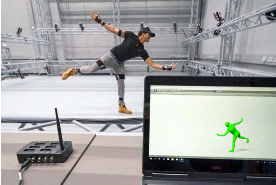
Figure 3.16: As few as six inertial measurement units worn on the body provide enough information to infer human pose. This makes motion capture practical in many scenarios.
