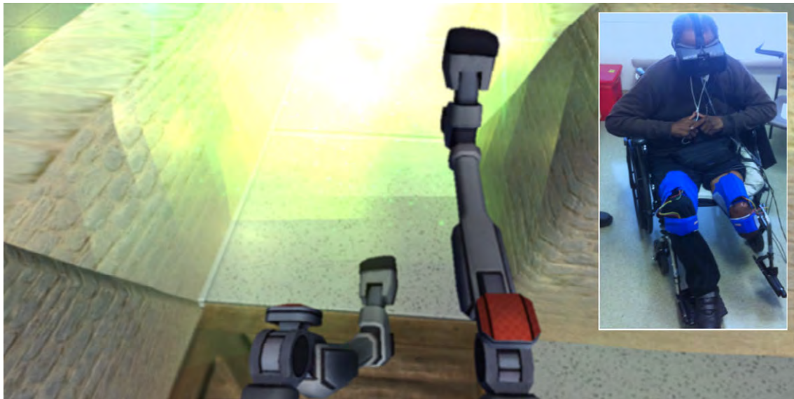
Figure 5.17: The right inset shows a lower-limb amputee using an early version of the created system. He wears an immersive VR headset and motion-tracking sensors on the upper and lower segments of both legs. The larger image shows his view of the virtual world, including the game scene and two intact legs that track the motions of his real legs.
