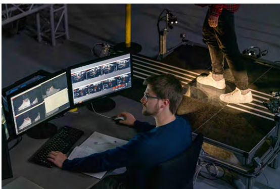
Figure 3.13: The 4D foot scanner captures a full 3D view of the foot during contact. The system images the bottom of the foot through a glass plate so that the deformation of the shape is captured. It is able to capture 4D sequences, revealing how feet interact with surfaces.
