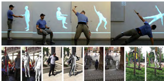
Figure 3.7: To take mocap out of the lab we use a small number of IMUs mounted on the body. Top: We train a neural network to regress full body pose from 6 IMUs. Bottom: We combine IMUs with a hand-held camera to obtain 3D poses in natural videos.
