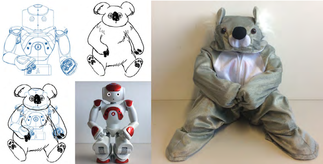
Figure 5.31: A conceptual design and initial prototype of the robot animal - a NAO robot enclosed inside a soft koala form.
