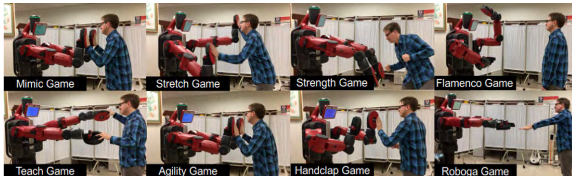
Figure 5.26: A user playing the exercise games with Max, our Baxter robot. The six games on the left involve physical interaction between the user and Max, whereas Flamenco and Roboga require motion but no contact.
