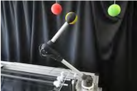
Figure 2.6: Muscle-based robotic arm serving as a testbed for Learning for Control. While it offers unique possibilities in terms of high accelerations, extreme speeds, and variable stiffness actuation, classical control methods are unable to unlock these abilities.
