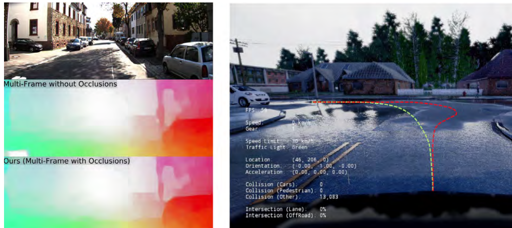
Figure 7.2: Understanding scenes in motions is crucial for intelligent systems. We have developed novel self-supervised approaches for learning optical flow from multiple images without ground truth (left). We have further developed a novel model for learning driving affordances from video sequences using limited supervision (right).
