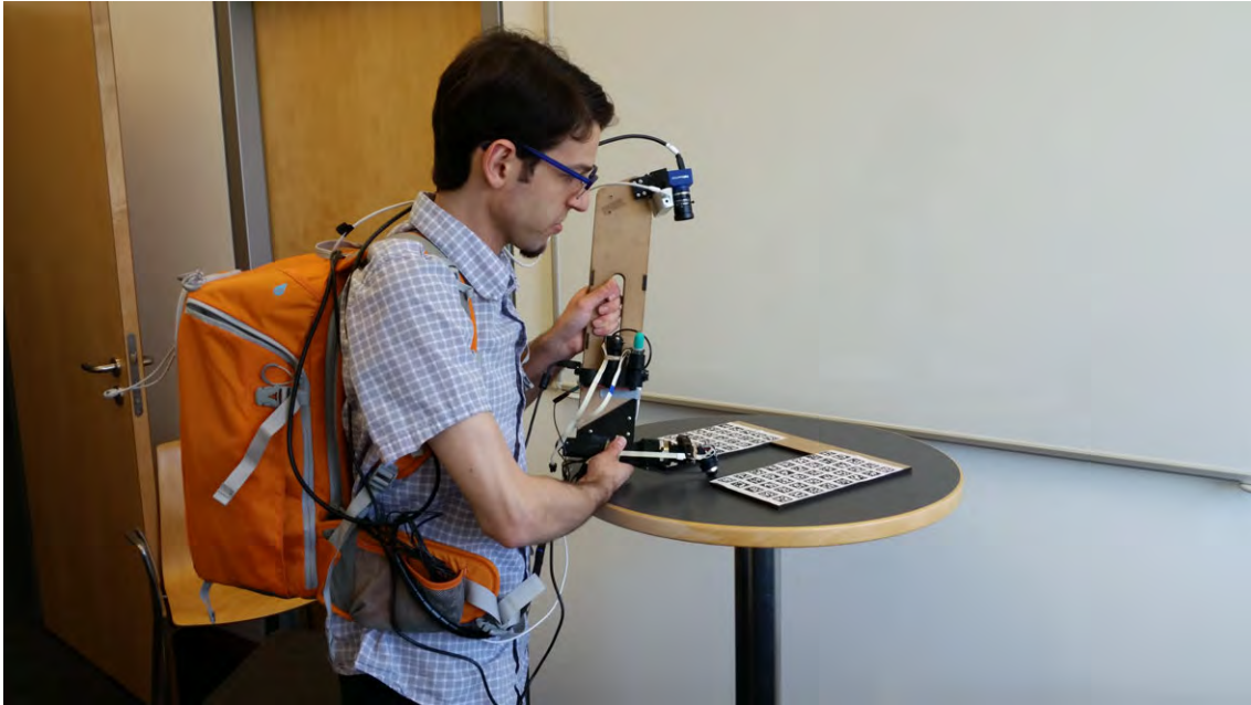
Figure 5.5: An experimenter operates the Proton Pack, a portable visuo-haptic surface interaction recording device.
