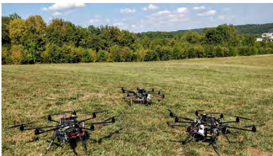
Figure 3.17: We have developed custom octo-copters with on board processing and cameras. These form the basis of our flying-motion-capture system, which aims to capture human and animal motion outdoors without any worn sensors.
