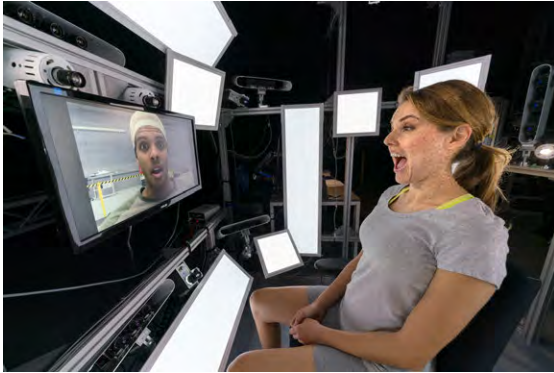
Figure 3.12: The 4D face and hand scanner captures detailed facial or hand shape at 60 fps together with high-quality texture.
