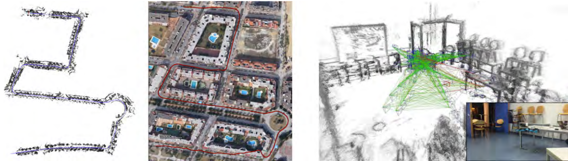
Figure 9.2: Left: Simultaneous localization and mapping with stereo vision and inertial sensing in an urban environment 6 . Right: Vision-based autonomous navigation of a multicopter using semi-dense monocular SLAM 7 .
