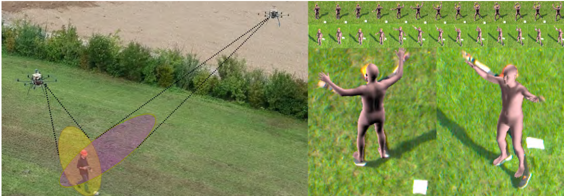
Figure 3.27: Two of our self-designed aerial robots cooperatively detecting and tracking a person on-board in real time (left). Cropped region of interests (ROIs) of images from both MAVs (right). The SMPL mesh with shape and pose estimated using our method is overlaid on all the images in a motion sequence.
