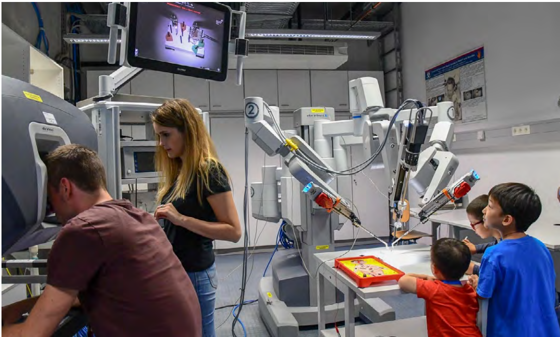
Figure 5.3: Paola Forte demonstrates her research to a visitor while three children look on. The Intuitive da Vinci Si surgical system that Paola uses in her research lets a doctor operate on a patient from across the room but normally provides no haptic feedback or other sensory augmentations for the operator.
