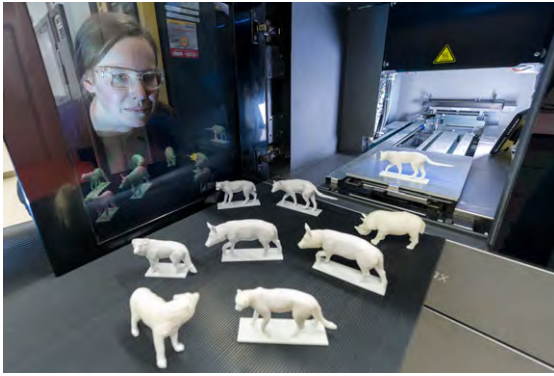
Figure 3.9: From a few snapshots of an animal, we reconstruct the detailed 3D shape. This can then be animated or 3D printed.
