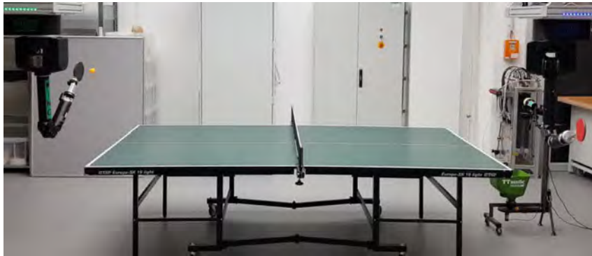
Figure 2.12: In the past, we have studied a single robot playing table tennis against a human or ball gun. In 2018, we migrated to a new lab and a setup with two robots. We aim to enable the unique high-speed Barrett WAM robot arms PING and PONG to jointly play table tennis in a collaborative game using methods from robotic skill learning.
