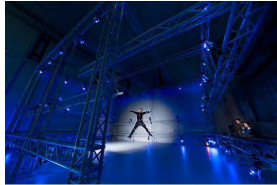
Figure 3.14: We recently added a 54-camera Vicon motion capture system to capture multiple people and complex motions.
